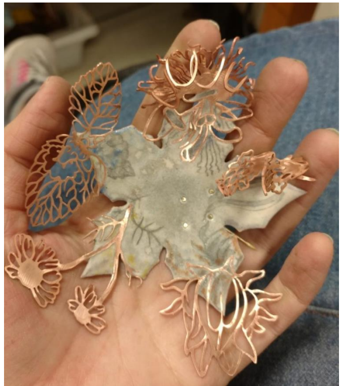
Figure 14: Enamel is applied, and graphite is sketched on
